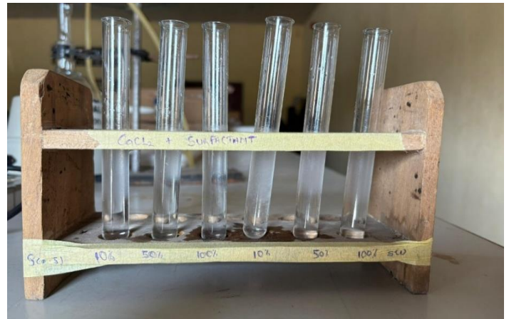
Figure 2: Visual observation of precipitation of \text{CaCl}_2 brines with SDS.
