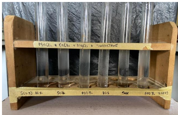
Figure 10: Visual observation of precipitation of NaCl+CaCl 2 +MgCl 2 brines with SDS.
